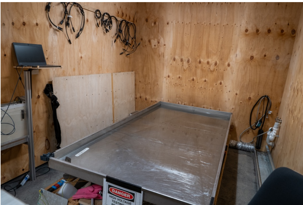
Figure 2: Wet Leakage testing bath at PV Lab
